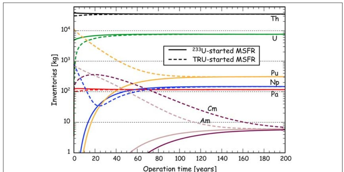
**Fig. 3** Evolution of MSFR core composition (kg/GWth). Solid lines correspond to a reactor started with  $^{233}\text{U}$  as fissile element while dash lines correspond to the case when the fissile elements are obtained from the TRU extracted from the waste of present LWR
