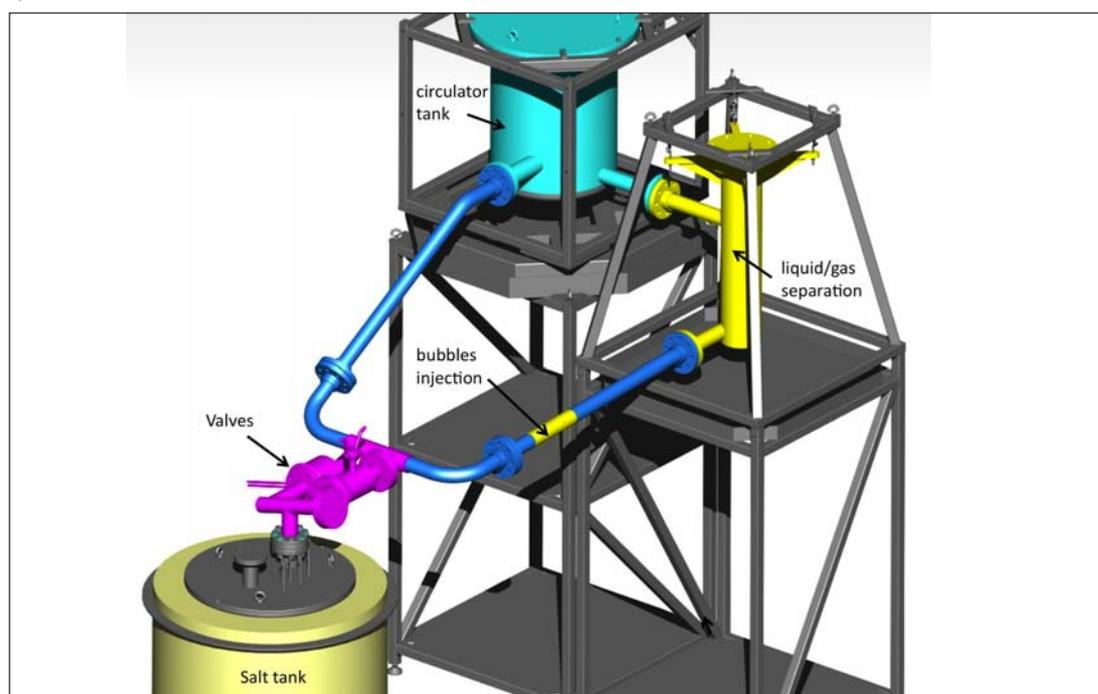
**Fig. 7** Simplified view of FFER facility under construction (CNRS, France). The loop is dedicated to bubbling studies and will work with a LiF-KF-NaF salt
