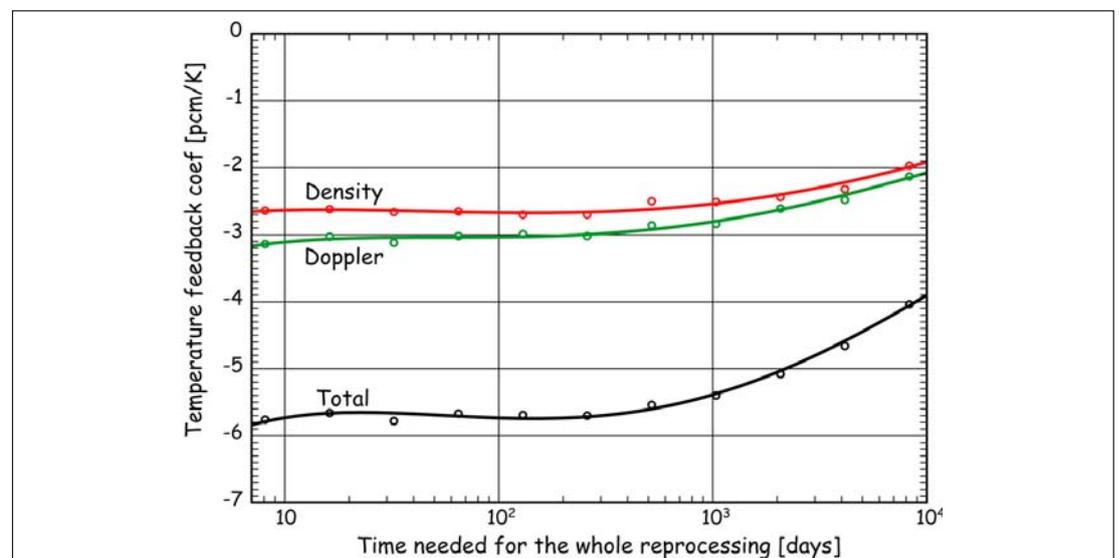
**Fig. 4** Feedback coefficients as a function of the reprocessing rate
