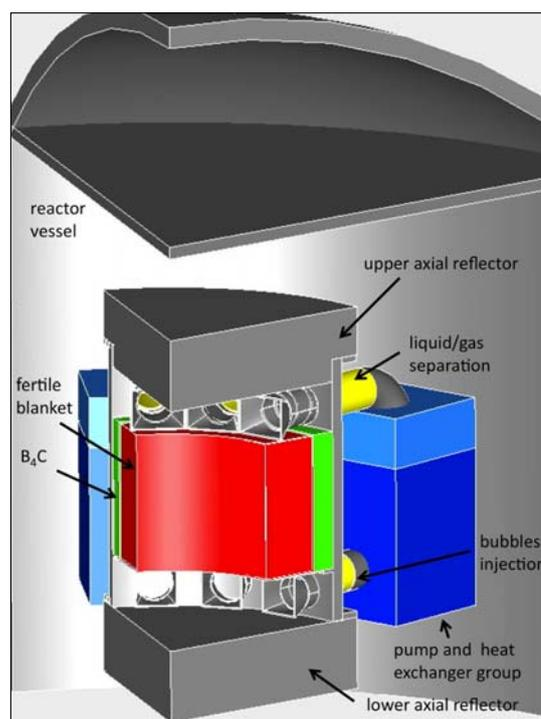
**Fig. 1. Schematic view of the MSFR general concept**
