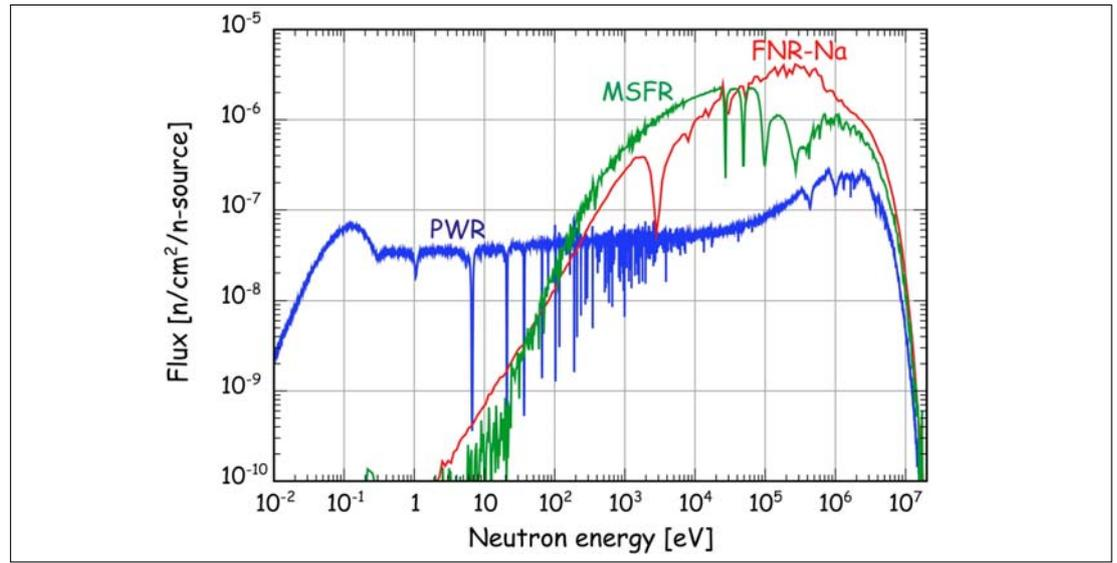
**Fig. 2** Fast neutron spectra of the MSFR and of a Na-cooled fast neutron reactor (FNR-Na) compared to the thermalized spectrum of a pressurized water reactor (PWR).
