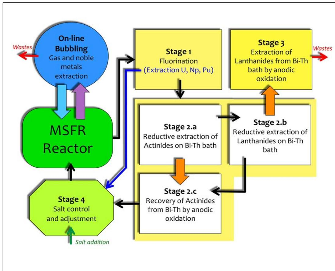
**Fig.5** Salt reprocessing scheme under investigation. Black or blue arrows indicate salt route, broad orange arrows point out transfers through lead-bismuth bath and broad blue/violet arrows transfers through gas
