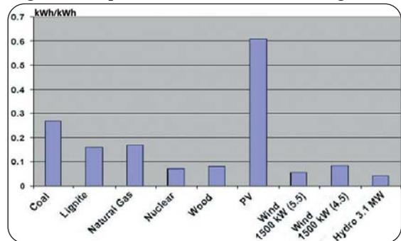
**Cumulated energy consumption (excluding fuel for operation) for various technologies** (Source University of Stuttgart)
