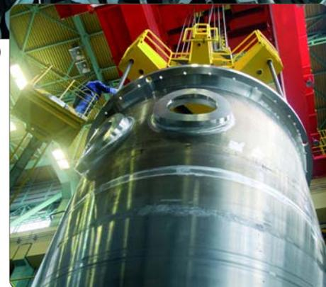
**Reactor Core Barrel (EPR)**
