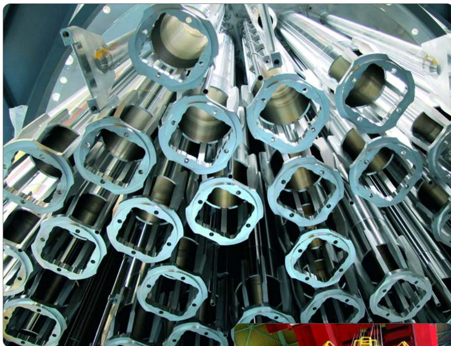
**Control Rod Guide Assembly (EPR Reactor Upper Internal Part)**
