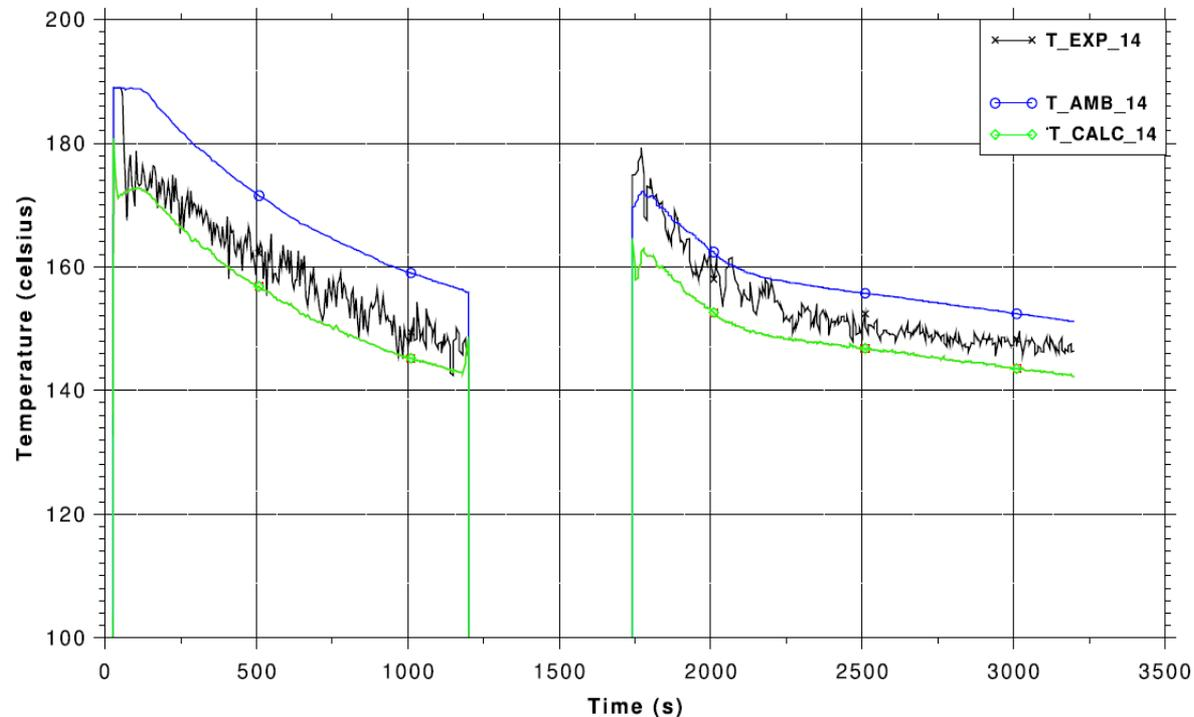
Measured (T\_EXP\_14) and calculated (T\_CALC\_14). Measured water temperature T\_AMB\_14 outside plume region.
