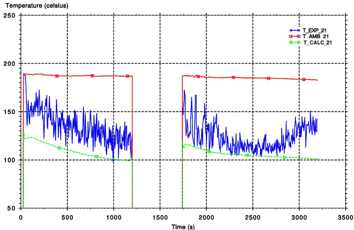
Measured (T\_EXP\_21) and calculated (T\_CALC\_21). Measured water temperature T\_AMB\_21 outside plume region.
