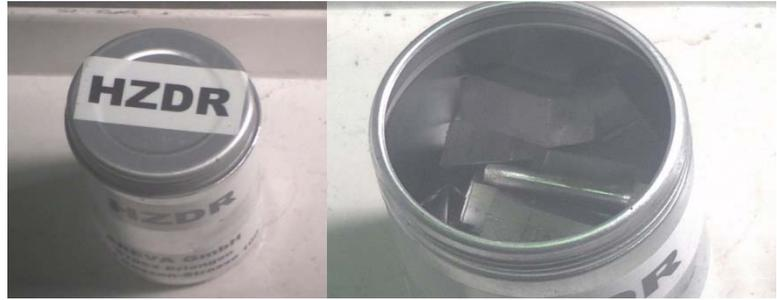
Figure 2: Transport can and irradiated specimens sent to HZDR Rossendorf
