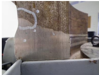
Fig.2: Test block with DMW for PAUT qualification
